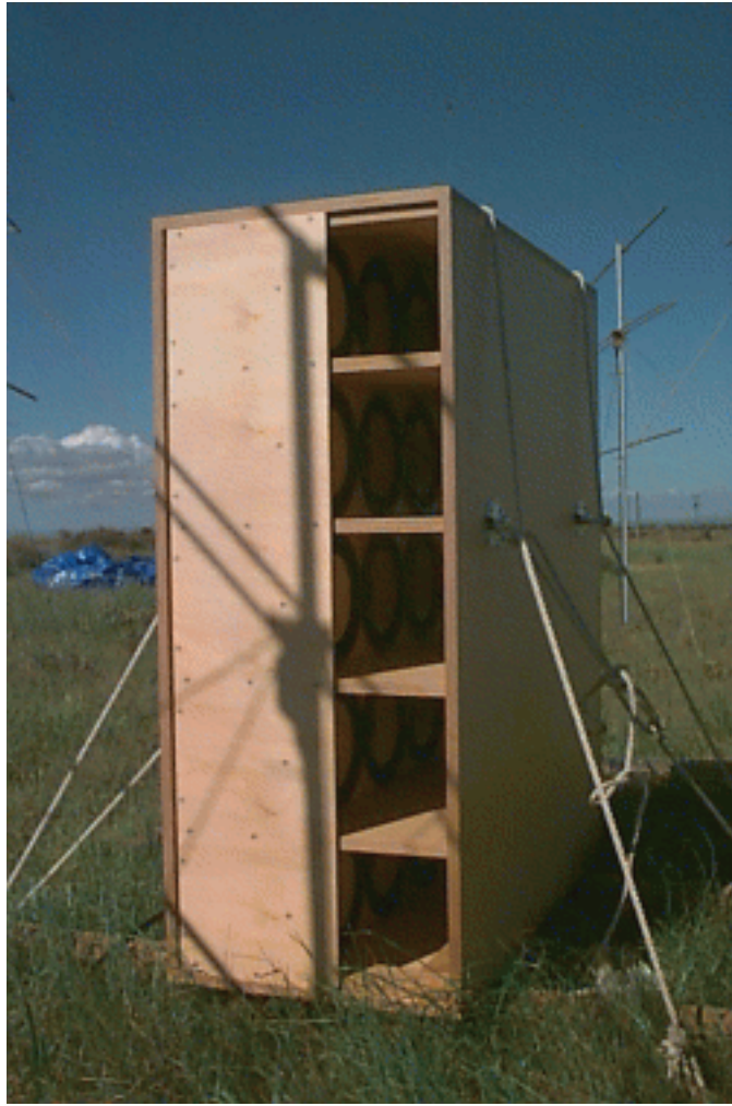
Figure 7.9: VAF E-115 RASS speaker at Buckland Park
