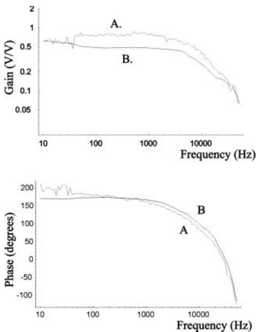
Fig. 6. The transfer functions for the low-frequency modulation port of the laser diode driver to the laser diode output (B) and the output of the injection-locked laser (A)
