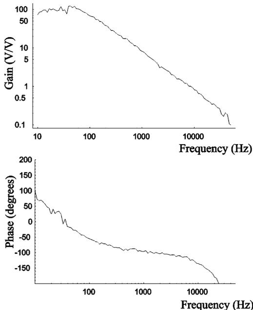
Fig. 8. The loop gain of the intensity noise reduction servo
