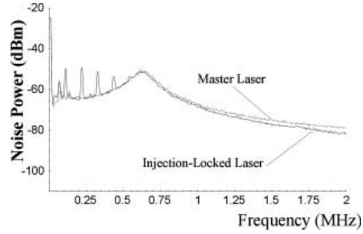
Fig. 10. The medium frequency intensity noise of the injection-locked slave and master laser. Measurement parameters: 9.5 mA photo-current, transimpedance gain = 500 V/A, detection bandwidth = 10 kHz, detector response = 0.7 A/W
