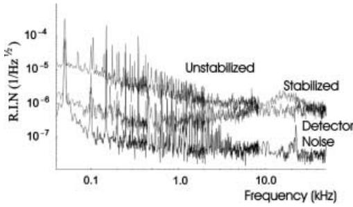
Fig. 9. Intensity noise reduction by feedback to the pump diodes of the slave laser
