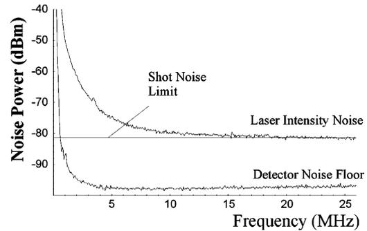
Fig. 11. High-frequency intensity noise with measurement parameters: photo-current = 46 mA, transimpedance gain = 500 V/A, detection bandwidth = 100 kHz, detector response = 0.7 A/W
