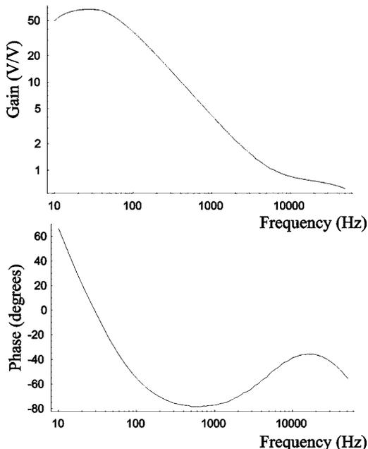
Fig. 7. The transfer function for the pre-amp used in the intensity noise reduction servo
