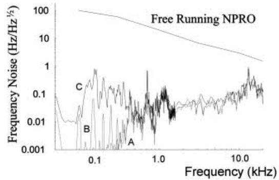
Fig. 4. A comparison of the predicted and measured contributions of the slave laser to the frequency noise of the injection-locked laser: (A) is the theoretical prediction, (B) is the contribution inferred from the PDH error signal and (C) is the frequency noise measured using the heterodyne technique
