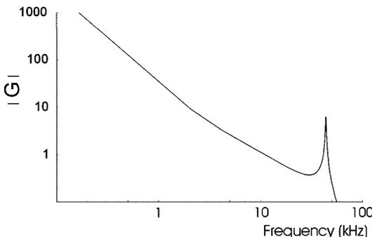
Fig. 2. The magnitude of the PDH servo loop gain
