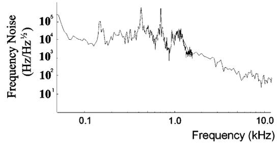
Fig. 3. The free-running frequency noise of the slave laser
