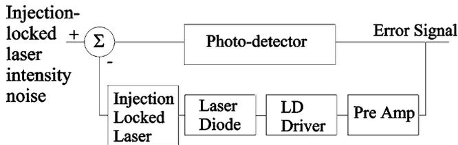
Fig. 5. A block diagram of the intensity noise reduction servo
