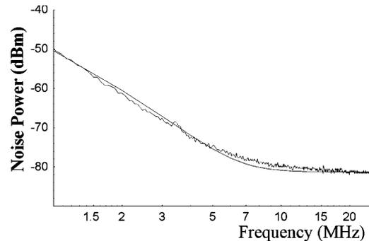
Fig. 12. A comparison of the measured intensity noise of the injection-locked laser and that predicted by (8). The measurement parameters are as for Fig. 11
