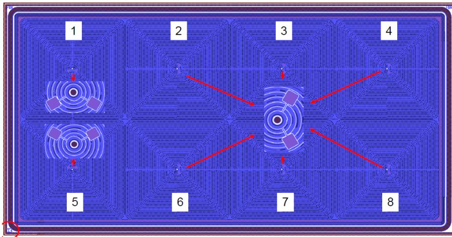
SDD-chip back side with bonding pads
