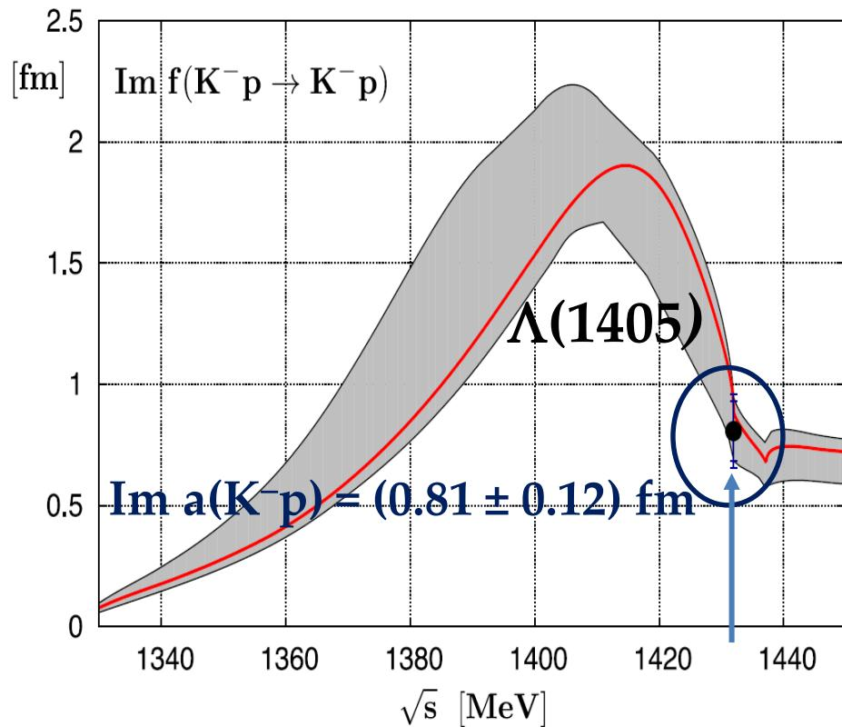
Real part (left) and imaginary part (right) of the  $K^- p \rightarrow K^- p$  forward scattering amplitude extrapolated to the subthreshold region, deduced from the SIDDHARTA kaonic hydrogen measurement.
