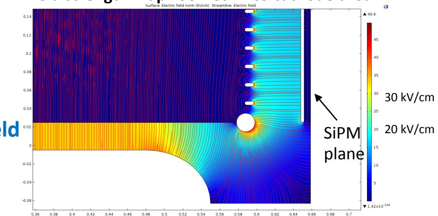
SiPMs plane in nEXO → Exposed to high electric field values.
