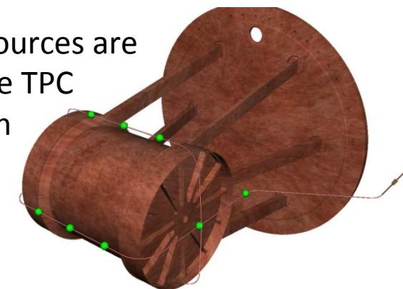
$^{228}\text{Th}$  is deployed every few days near the cathode to monitor the  $e^-$  life time and measure the energy response.
