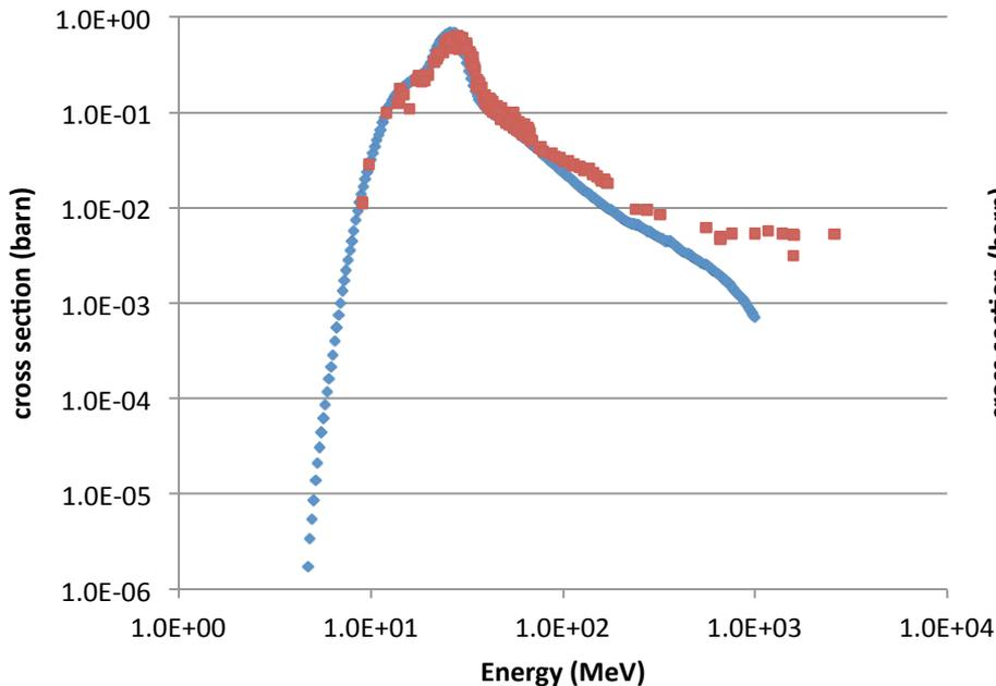
cross section  ${}^{\text{nat}}\text{Pb}(d,x){}^{206}\text{Bi}$
