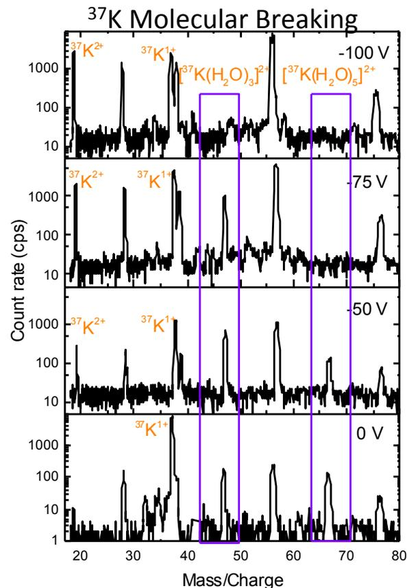
$2^+$  molecular ions breaks and  $^{37}\text{K}^{2+}$  produces when offset voltage increases.
