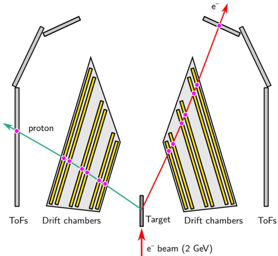
We detected the lepton and proton in coincidence.
