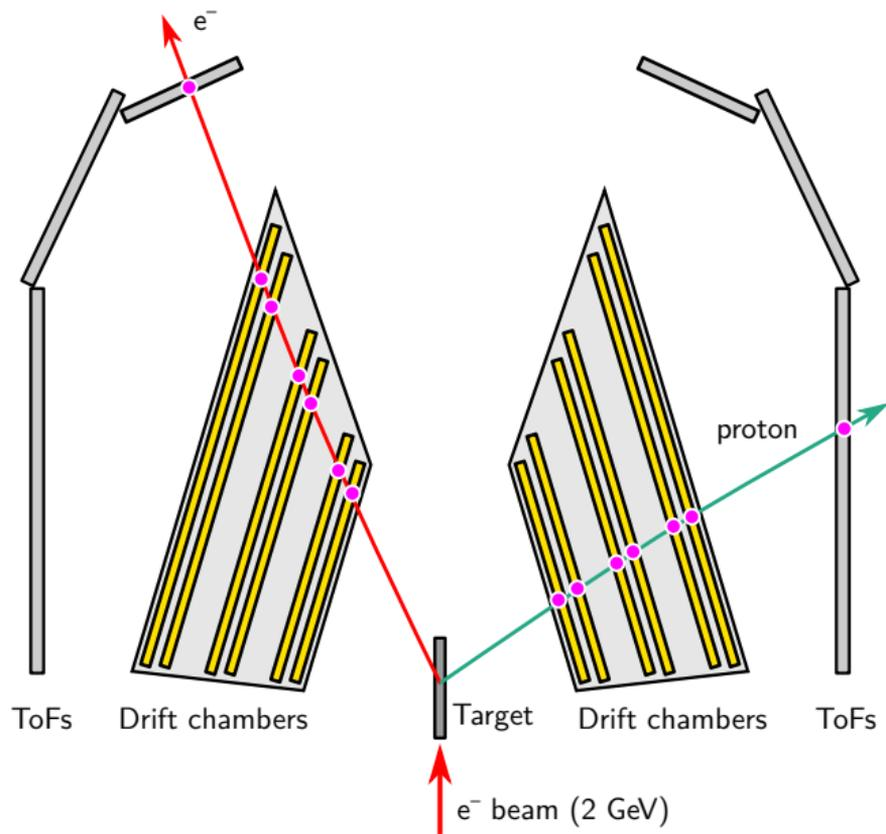
We detected the lepton and proton in coincidence.
