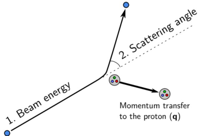
Elastic scattering kinematics are fixed by two parameters.
