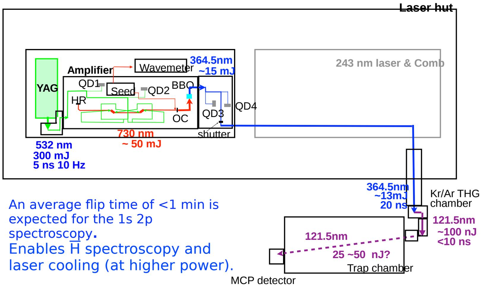
An average flip time of <1 min is expected for the 1s 2p spectroscopy.
