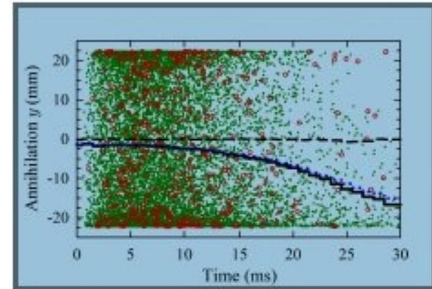
Annihilation locations: The red circles are the annihilation times and y-locations for 434 real anti-atoms, as measured by our particle detector. The green dots are from a simulation of  $\bar{H}$  with 100X the H mass. Black solid line is  $\langle y \rangle$ .
