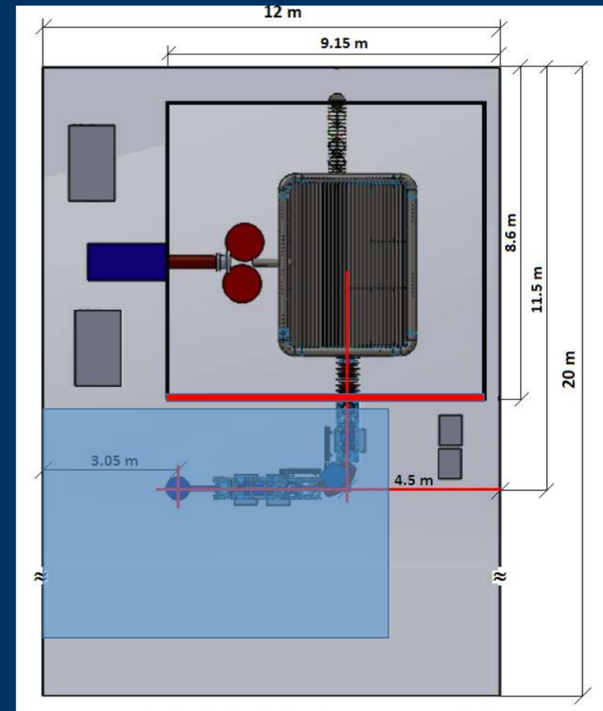
Accelerator floor plan
