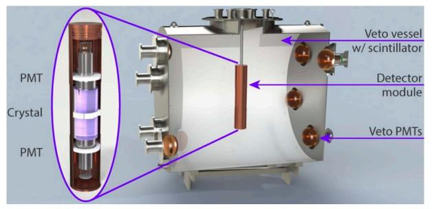
**Proof of principle** (LNGS): 5-kg ultra-low background NaI(TI) **Veto system:** 1.4m diam, 1.5m length, LAB liquid scintillator **Full detector** (LNGS & SUPL): ~50kg @ each site
