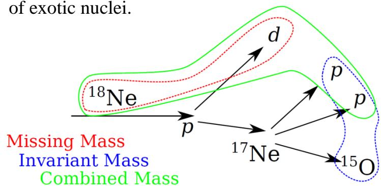
Combined mass spectrum of  $^{17}\text{Ne}$  measured by the Acculinna provided a limit  $\Gamma_{2p}/\Gamma_\gamma < 8 * 10^{-5}$  [ P. Sharov et al., talk given at EXON2016 ].
