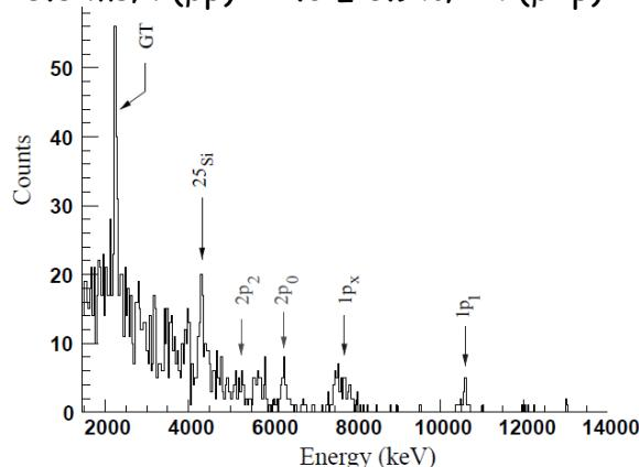
**Fig.** Charged-particle spectrum of the decay of  $^{27}\text{S}$  nuclei implanted in the E3 silicon detector. Proton groups above about 7 MeV have to be reconstructed by summing the energy signals from detectors E3 and E4.
