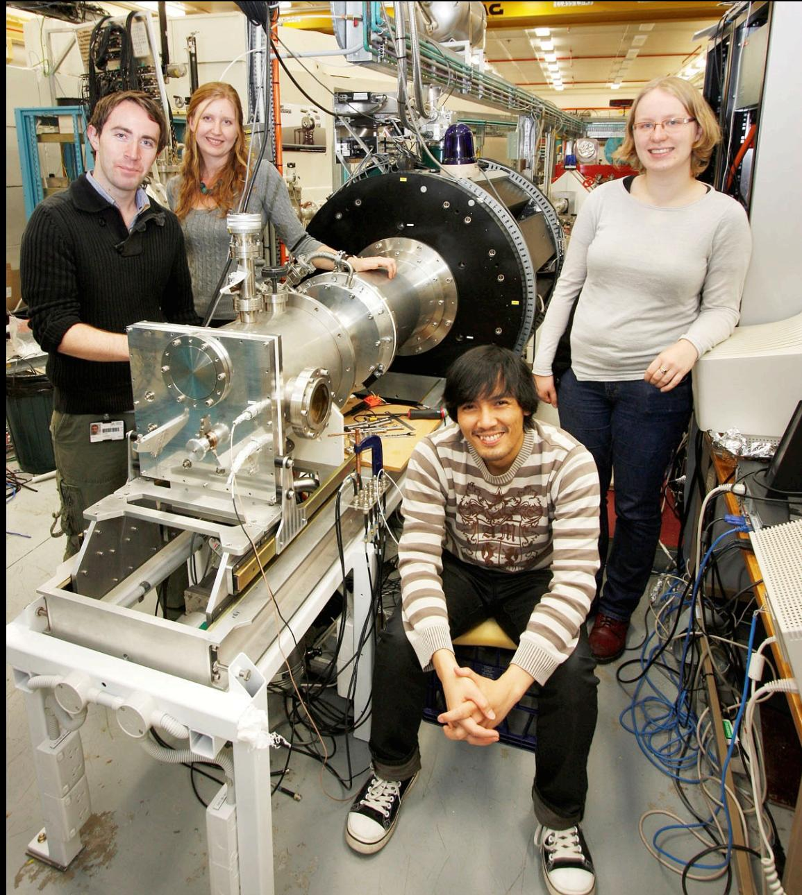
RIB: SOLEROO 6.5T s/c solenoid and tracking detectors
