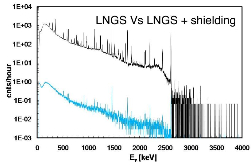
Passive shielding is more effective underground since the  $\mu$  flux, that create secondary  $\gamma$ s, is suppressed.
