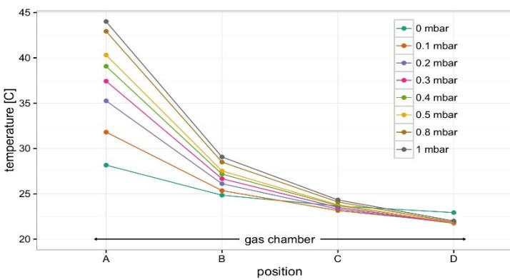
Temperatures have been measured along the gas chamber (only)
