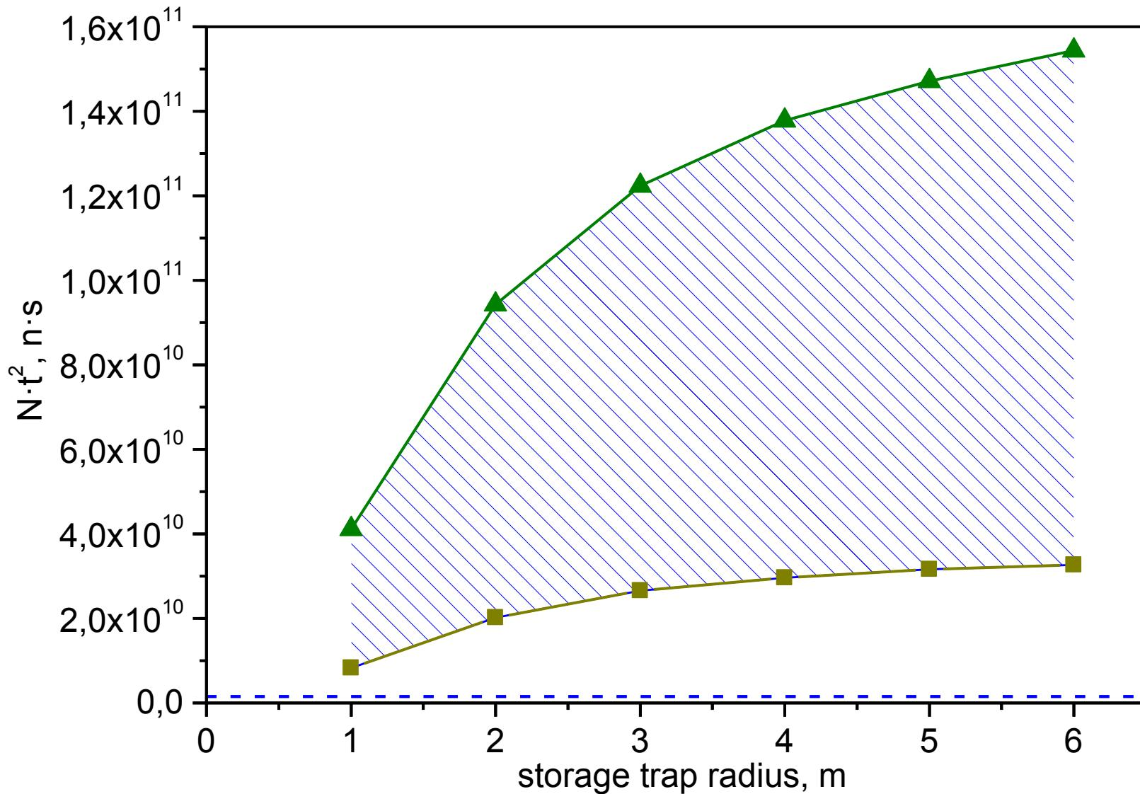
Storage trap: height 2.5 m,  $v_{\text{boundary}} = 6.8 \text{ m/s}$ , diffusion 90 %, abs. in walls  $3 \cdot 10^{-5}$
