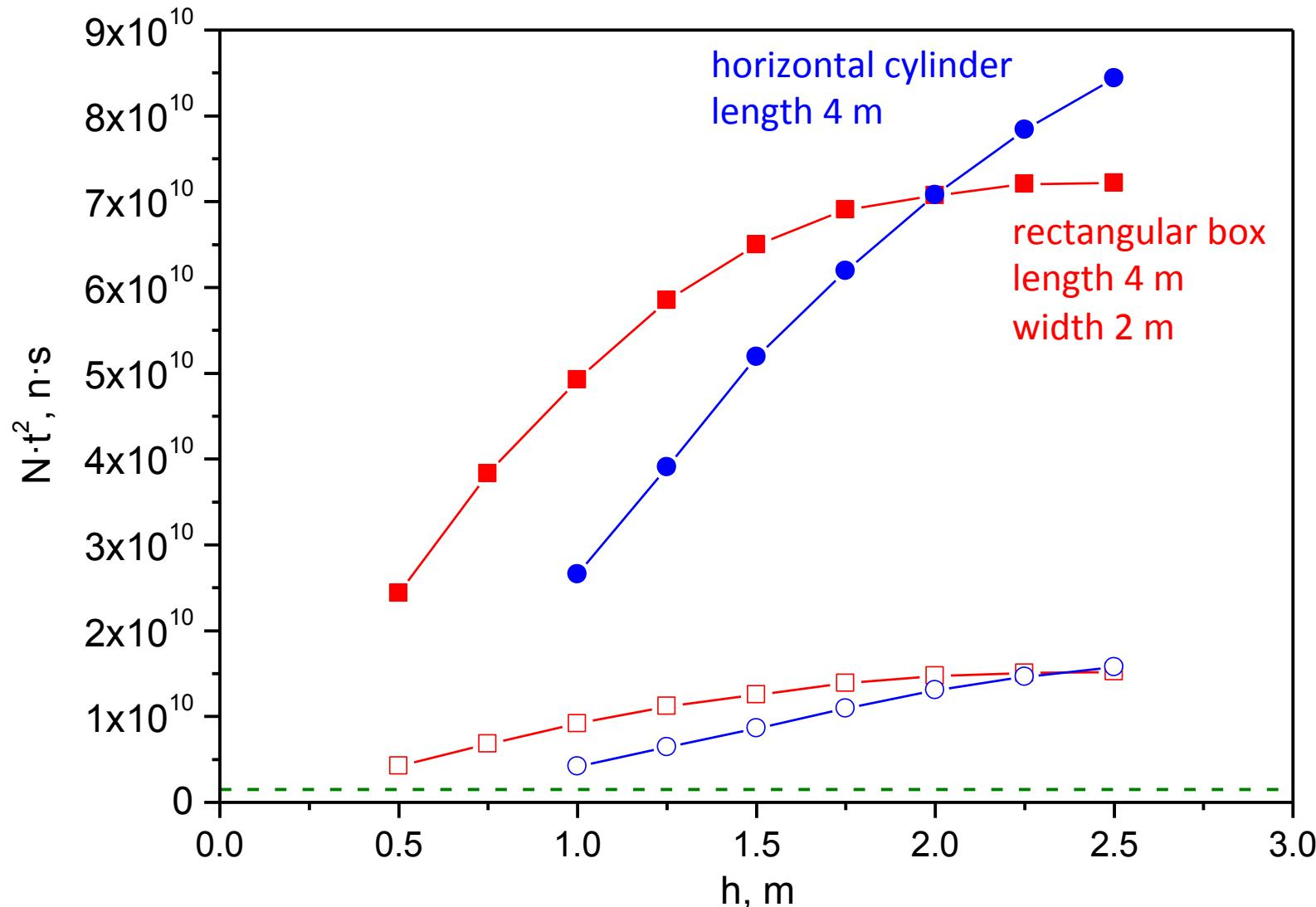
Storage trap:  $v_{\text{boundary}} = 6.8 \text{ m/s}$ , diffusion 90 %, abs. in walls  $3 \cdot 10^{-5}$
