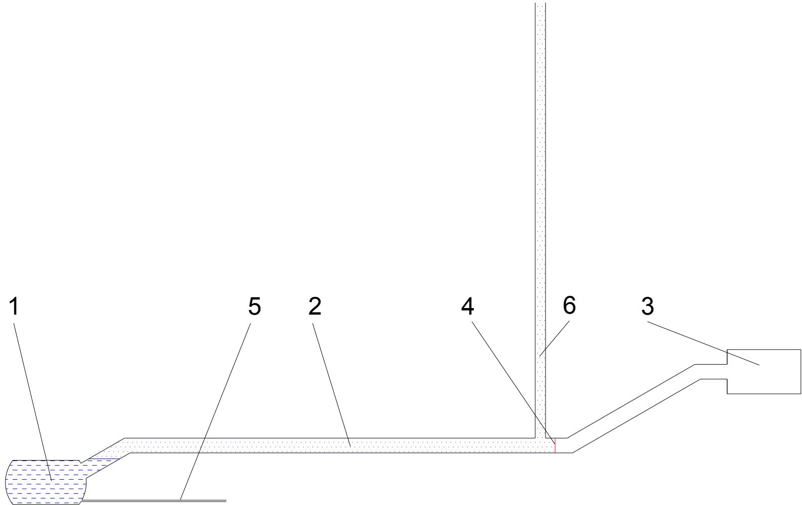
(1) source chamber; (2) neutron guide; (3) UCN trap; (4) membrane in front of the inlet to the UCN trap;(5) pipe for filling the chamber; (6) pipeline for evacuation of the chamber (UCN gravitational shutter)
