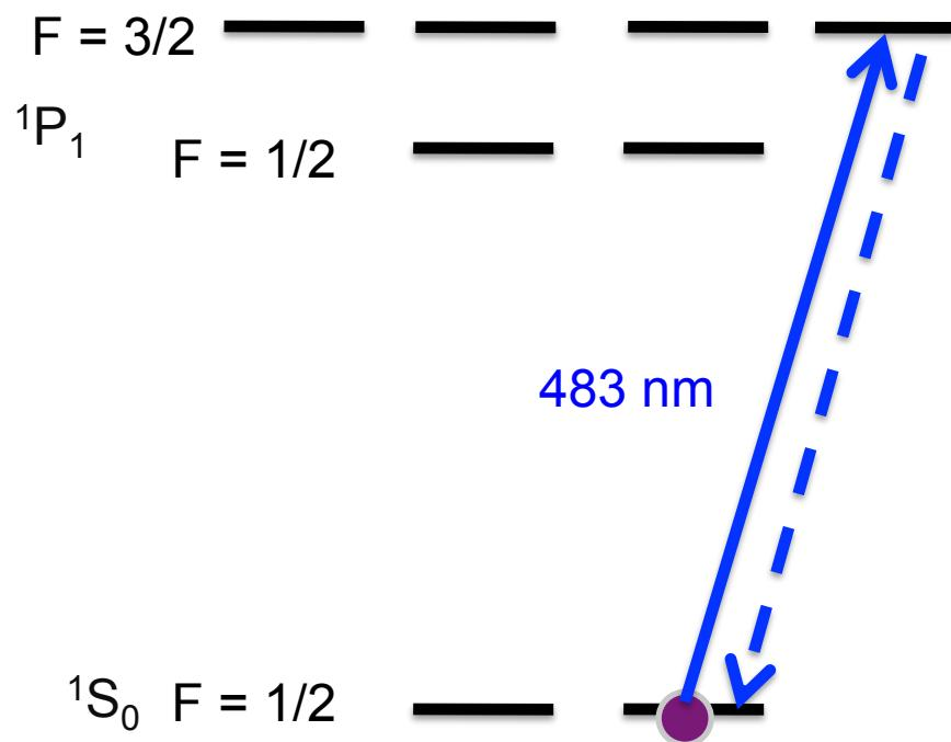
Increase from 2.5 photons per Atom to 1000 photons per atom, For a nominal SNR improvement of 20.
