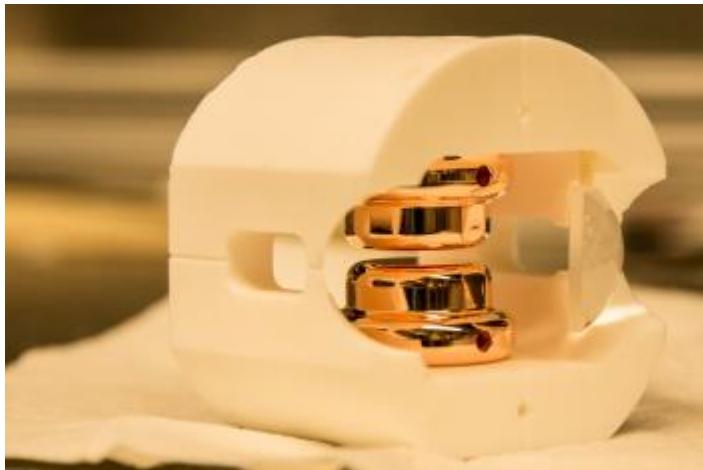
Present: Copper Electrodes,  $E = 70 \text{ kV/cm}$
