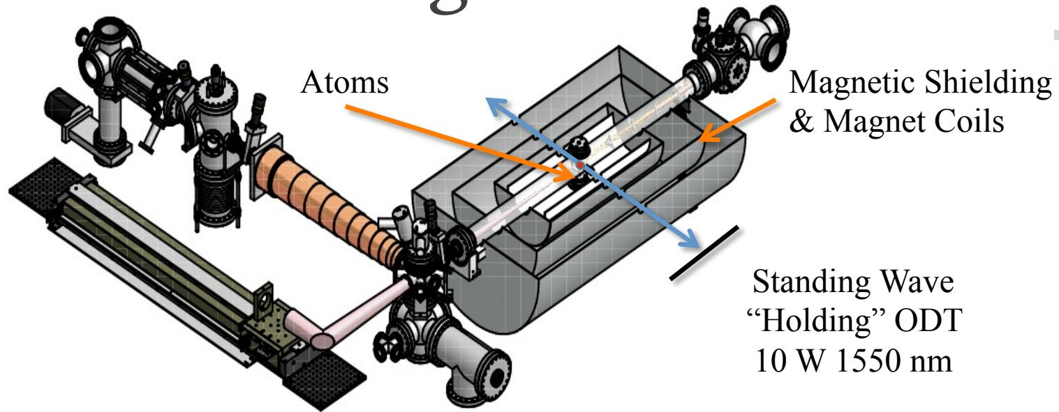
ODT→ODT Transfer: 70% Efficiency
