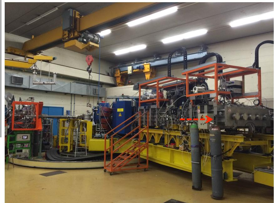
PRISMA magnetic spectrometer
