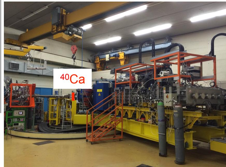
PRISMA magnetic spectrometer
