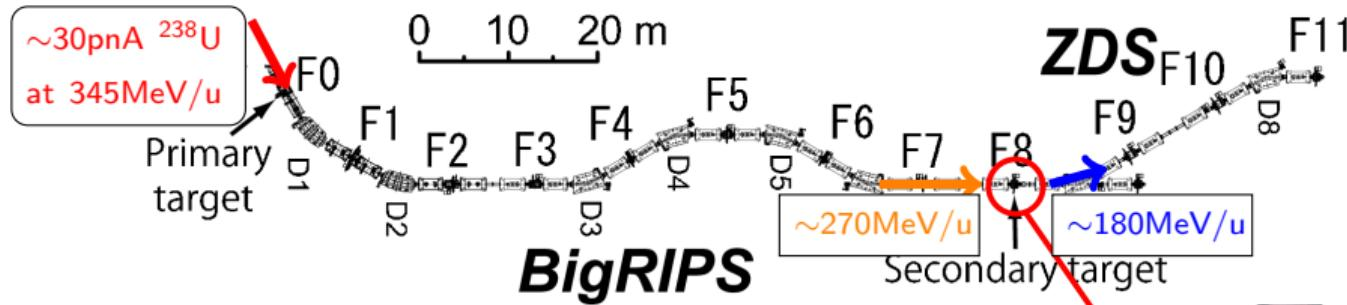
Secondary Target: 100 mm liquid hydrogen
