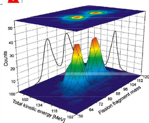
330 fission events were identified and the mass of the fragments determined from energy loss measurements using two silicon detectors
