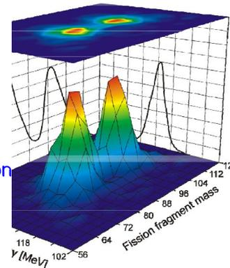
330 fission events were identified and the mass of the fragments determined from energy loss measurements using two silicon detectors
