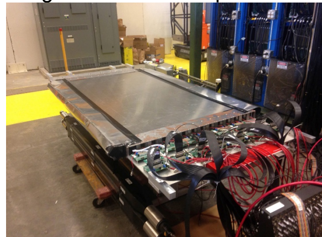
UVa High rate X-ray testing setup for GEMs
