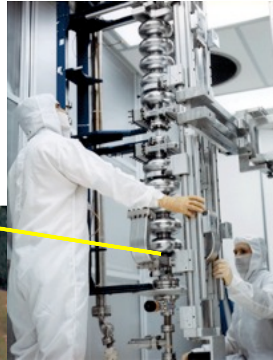
Superconducting radiofrequency (SRF) cavities undergo vertical testing.
