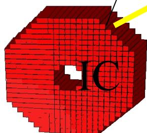
Inner Calorimeter (424 PbWO<sub>4</sub> crystals) to detect high energy photons at forward lab angles.
