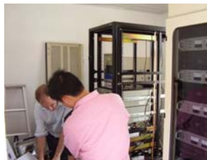
Figure 6. (Left) Photograph showing the transmitter (right of the image) and receiver rack being assembled (left of image).
