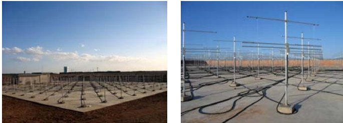
Figure 2a (left): Photograph of the Jiuquan Wind Profiler in China with the launch facilities in the background. There are 144 Yagi antennas arranged on a square grid. The radar equipment is housed in the building to the centre left of the image. Figure 2b (right): The Jiuquan VHF radar, showing the antenna array. The individual antennas are three element Yagis with a folded dipole driven element. The basic array square grid spacing is \lambda/\sqrt{2} , which makes the largest inter-antenna distance \lambda . This ensures that there are no grating lobes associated with the array polar diagram. There are 36 feeds into the array. These are split into 4 separate feeds which then drive 4 separate individual antennas. This arrangement is shown schematically in Figure 3 below. The radar beamwidth is about 7° and the 5 radar beams are directed E, W, N, S and vertical at 15° off-zenith in sequence. The array dimensions are given in wavelengths. For frequencies near 50 MHz the array dimension is about 50 m on edge.
