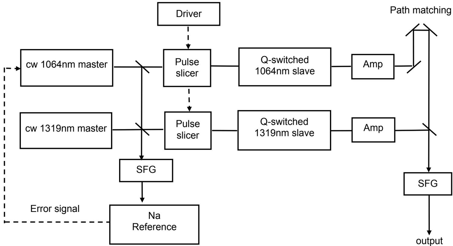
SFG (1064 nm + 1319 nm  $\rightarrow$  589 nm) uses single-pass LBO
